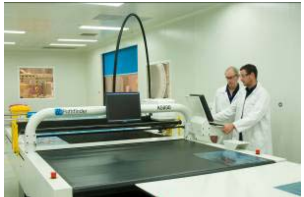
Quickstep team members Sean Scammell and David Howarth operating Quickstep's new Ply Cutting machine
