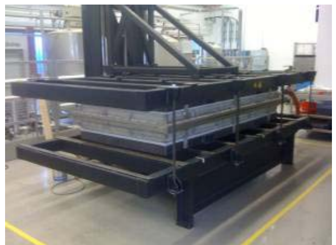
Quickstep’s curing chamber in operation at Quickstep’s German facilities
