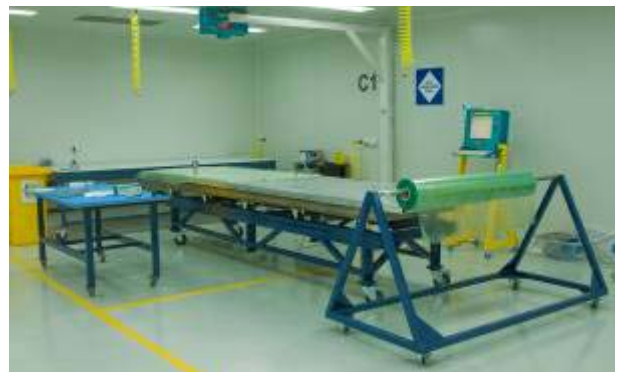
Ply Projection Equipment in operation in Quickstep's new clean room
