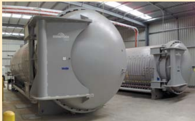
The 2 Bondtech Autoclaves giving Quickstep second largest aerospace grade curing capacity in Australia second only to Boeing in Victoria.
