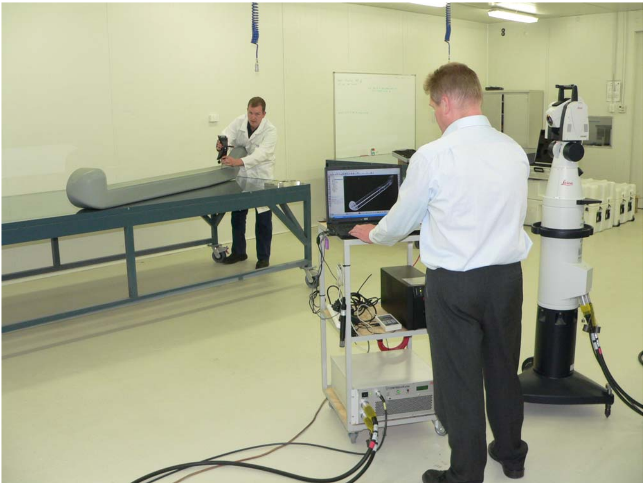
A Leica Laser Tracker, recently installed at Quickstep's Fremantle manufacturing site, used for aerospace parts manufacturing.
